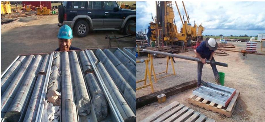
Solid cores laying in core trays taken from Kelly1 well site at approx 611m. Taking solid cores from the core barrel.
