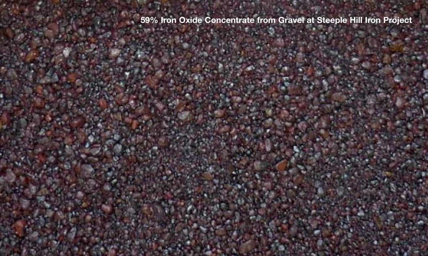
59% Iron Oxide Concentrate from Gravel at Steeple Hill Iron Project
