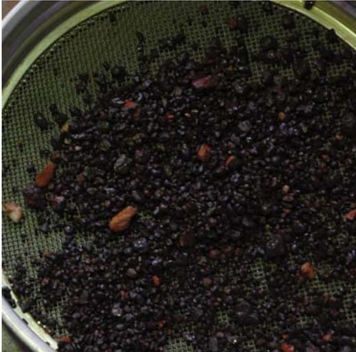
Plate 1: Washed Iron Ore detritals in sieve
