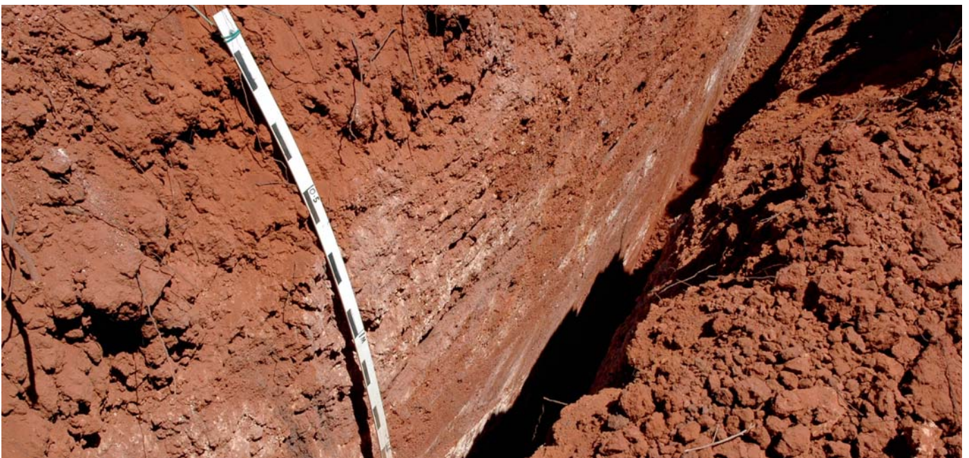
Plate 1: Pit 077 with Alluvium to 0.7m, then Iron Oxide rich gravel to 3.5m
